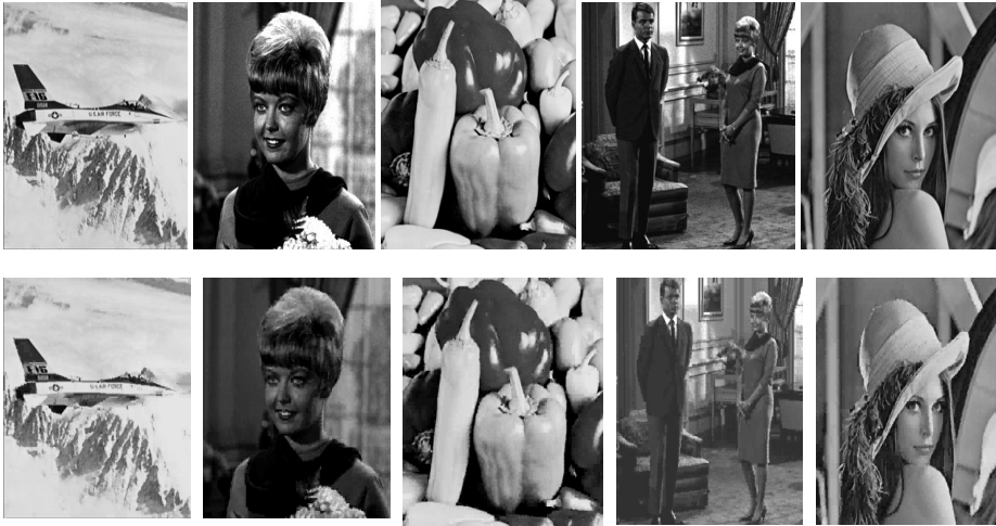
Fig. 2. Original images and reconstructed images with compression ratio = 0.500 bpp using the CCHNN algorithm: (row 1) are original images; (row 2) are reconstructed images with codebook of size k = 256 .
